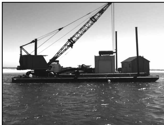
The Barnstable County dredge arrived in mid-April and dumped 9,000 cubic yards from the outer channel onto the Spit.
